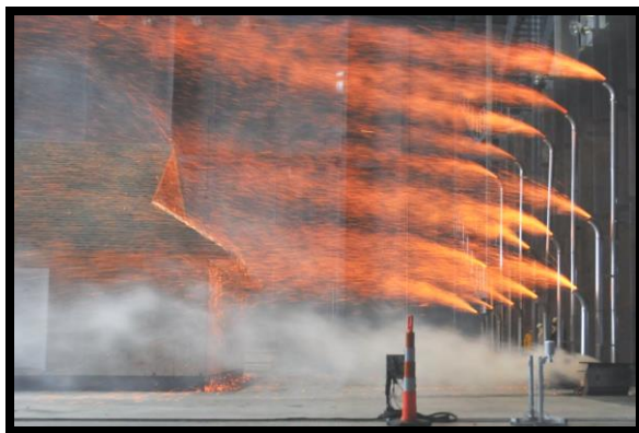
Ember intrusion testing by the Institute for Business & Home Safety. Learn more at: http://www.disastersafety.org/
