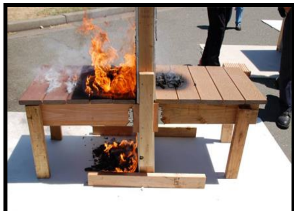
Firebrand testing on various decking material products. For more information visit: http://firecenter.berkeley.edu/
